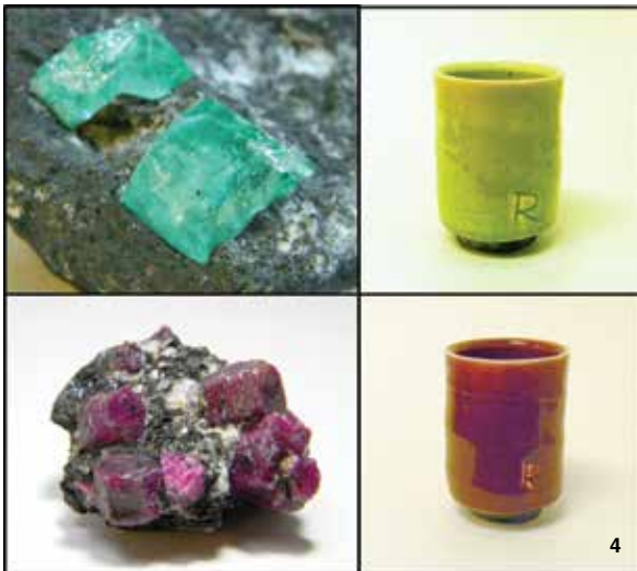
4 Emerald and ruby, left, and the corresponding Emerald/Ruby glaze with chromium oxide (top right) and chromium oxide with 6% tin oxide (bottom right). Note: All of the color sample yunomi were made with Laguna cone 6 Frost porcelain. All images of gemstones samples: Courtesy of the Lora Robins Gallery of Design from Nature.
