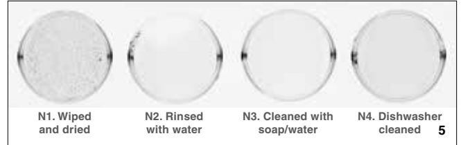
2 Dissection microscope (center) and SEM images (left) of a tile with a crazed glazed surface, showing craze lines and fissures. 3 Bacterial survival results of increasingly stringent washes on a crazed glaze surface. 4 Dissection microscope (center) and SEM images (left) of a tile with a non-crazed glaze surface, showing surface pores and defects. 5 Bacterial survival results of increasingly stringent washes on a non-crazed glaze surface.
