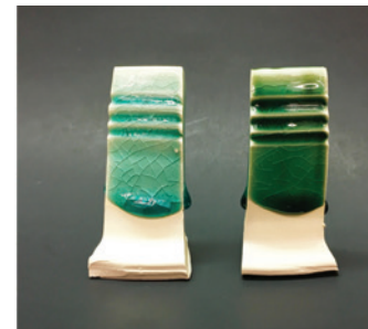
Figure 8: Color profile of copper carbonate. Samples show increasing concentration from left to right.
