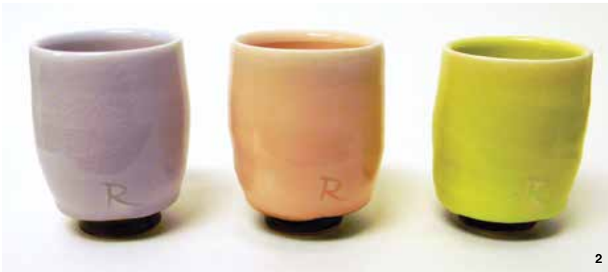
1 Test tiles with Bubble Base glaze. Colorant additions from Left to right: Neodymium Oxide, erbium oxide, and praseodymium oxide. 2 From left to right: A yunomi with WTF Purple glaze, a 7% neodymium oxide glaze; a yunomi with Sorority Pink glaze, an 8% erbium oxide glaze; a yunomi with Nucular Green glaze, a 7.5% praseodymium oxide glaze. 3 A yunomi with WTF Purple glaze photographed under three different light sources. From top to bottom: halogen light bulb, incandescent light bulb, and LED light bulb. All yunomi prepared with cone-6 Laguna Frost porcelain and fired to cone 6 in oxidation.
