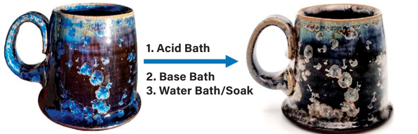
3 Acid-etching of a copper-oxide crystalline surface through the process described below, in which copper is pulled out of the crystals seen at left to make the lighter colored ones seen at right. 4 A crystalline glaze with 7.5% manganese oxide and 2% cobalt oxide, in which the cobalt is preferentially leached out of the crystals (left)—to make silver crystals with gold rings over a black background (right).
