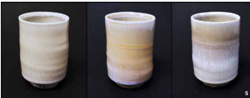
5 Sample cups with the Mid-Range Glaze Base with different additions to help isolate the effects of various components of rutile. From left to right, 3.5% titanium dioxide/0.5% black iron oxide blend; a 1% Nb addition; followed by 4% light rutile in the same glaze base.
