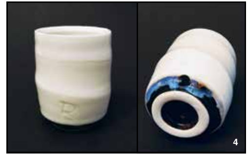
3 Niobium oxide was added to the Mid-Range Glaze Base (at 1, 2, and 3%) and fired to cone 6 in oxidation (left) and cone 10 in reduction (right). 4 Yunomi, Laguna cone 6 Frost porcelain, 1% niobium glaze, fired in oxidation. The opalescence is visible on the oxide-washed band near the foot.
