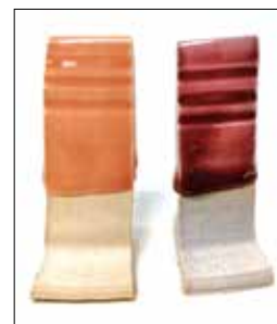
1 Roughly 40 milligrams (0.0394 grams) of gold chloride, suspended in a 100-gram sample of Ron Roy's clear base, and fired to cone-6 oxidation, left, and cone-10 reduction, right.
