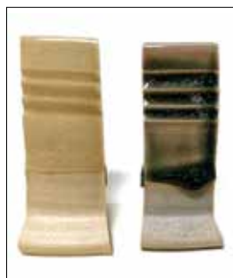
3 Color results from 0.50 grams of silver nitrate, suspended in a 100-gram sample of Ron Roy's clear base, and fired to cone-6 oxidation, left, and cone-10 reduction, right.
